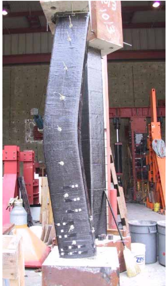
Posttest Flexure-Membrane Response
