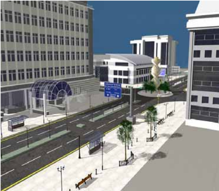
Anti-ram bollards blended with the street furniture.
