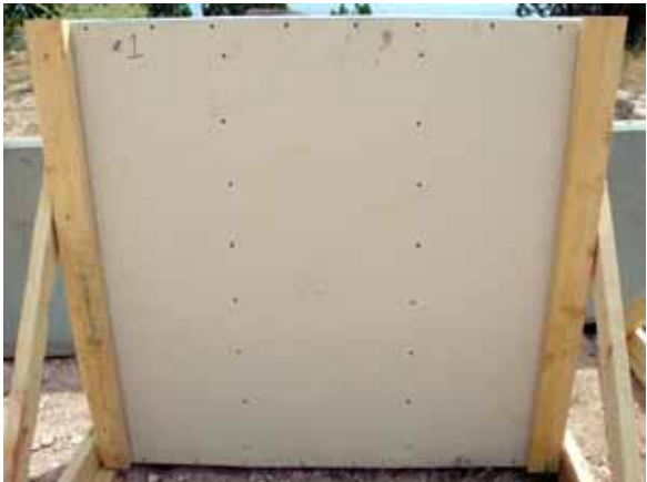
Rear Face of Wall (No Perforation Occurs)
