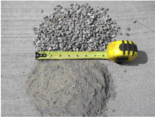
Interstitial Fill Between Studs Used to Stop Ballistic Perforations
